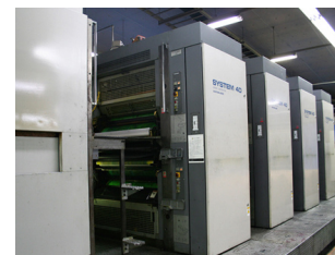
A state-of-the-art waterless offset rotary press. High resolution printing achieved with the help of Vulcan blankets
