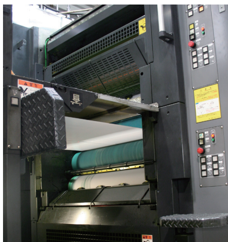
A Vulcan Alto ND2 blanket installed on a horizontal offset rotary press
