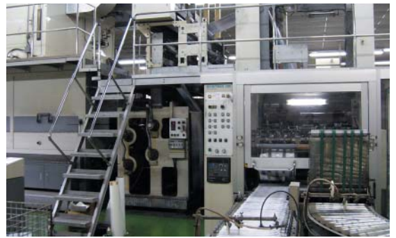
An offset rotary press at the Nishikawa Printing headquarters factory equipped with Vulcan offset printing blanket, one of six offset rotary presses in its two factories.
